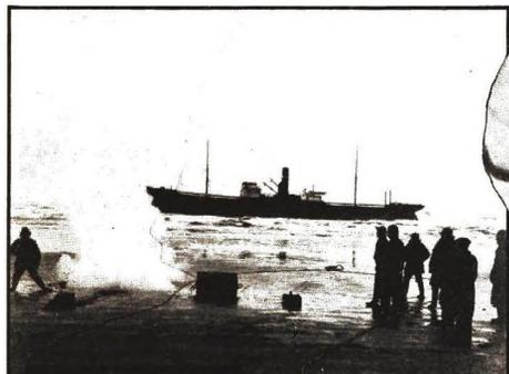
Above and left: The Lyle gun shoots a line 700 yards. To the shot line is attached a sturdy three-inch rope which bears the weight of the breeches buoy.
